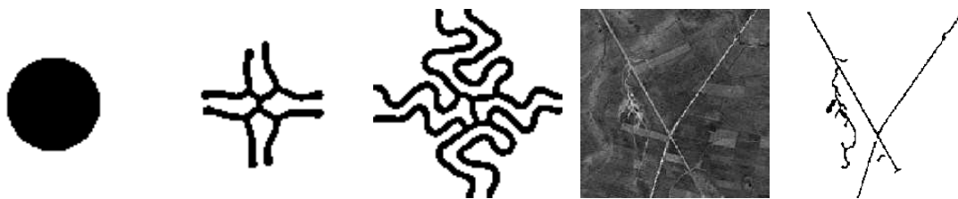
Figure 13. Three leftmost images: the evolution of a circle under non-local forces, showing the development of a reticular structure. Second to right, a satellite image and right, the result of road network extraction.
