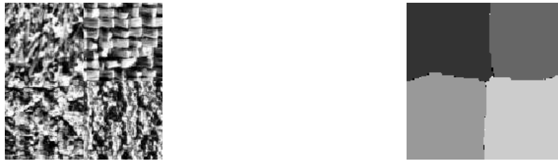
Figure 10. A texture mosaic and the result of the wavelet-based level set classification.
