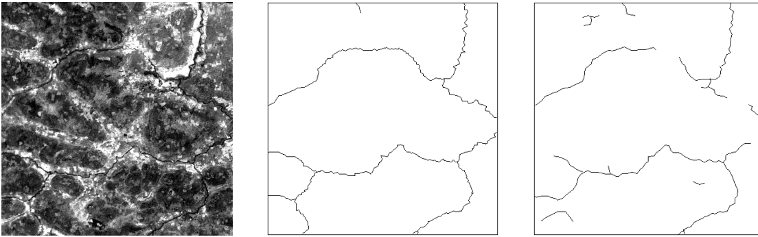
Figure 7. Results of line network extraction from a satellite image (SPOT XS2) of size 682 \times 674 pixels. On the left is the data image, in the center the reference line network, manually extracted by an expert (BRGM), and on the right is the extracted line network.
