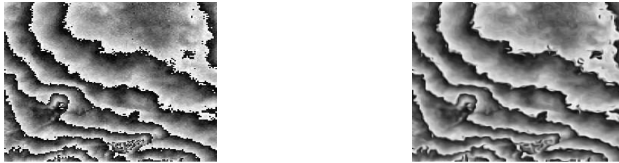
Figure 14. Left: interferogram data from part of Utah; right: the filtered result after 30 iterations.
