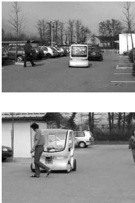
Figure 8. An experimental setting showing the execution of a pre-planned trajectory among pedestrians and unaccounted for vehicles.
