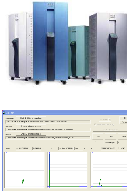
Figure 15. AMIB-E P1: a first prototype tool for preventive maintenance of UPS electronic components.
