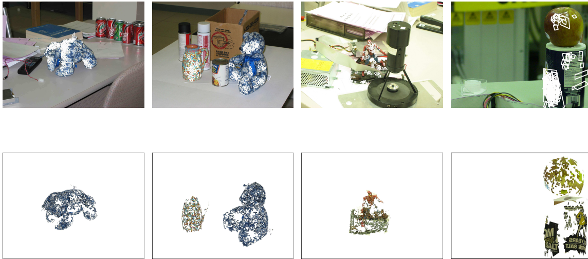
Figure 5. Object recognition experiments. The top row shows the model patches that were matched to the images, and the bottom row shows the models recognized, rendered in their estimated poses. Note that the teddy bear in the leftmost column is in a pose radically different from those used to acquire its model, and that there is a significant amount of clutter and occlusion in each image.
