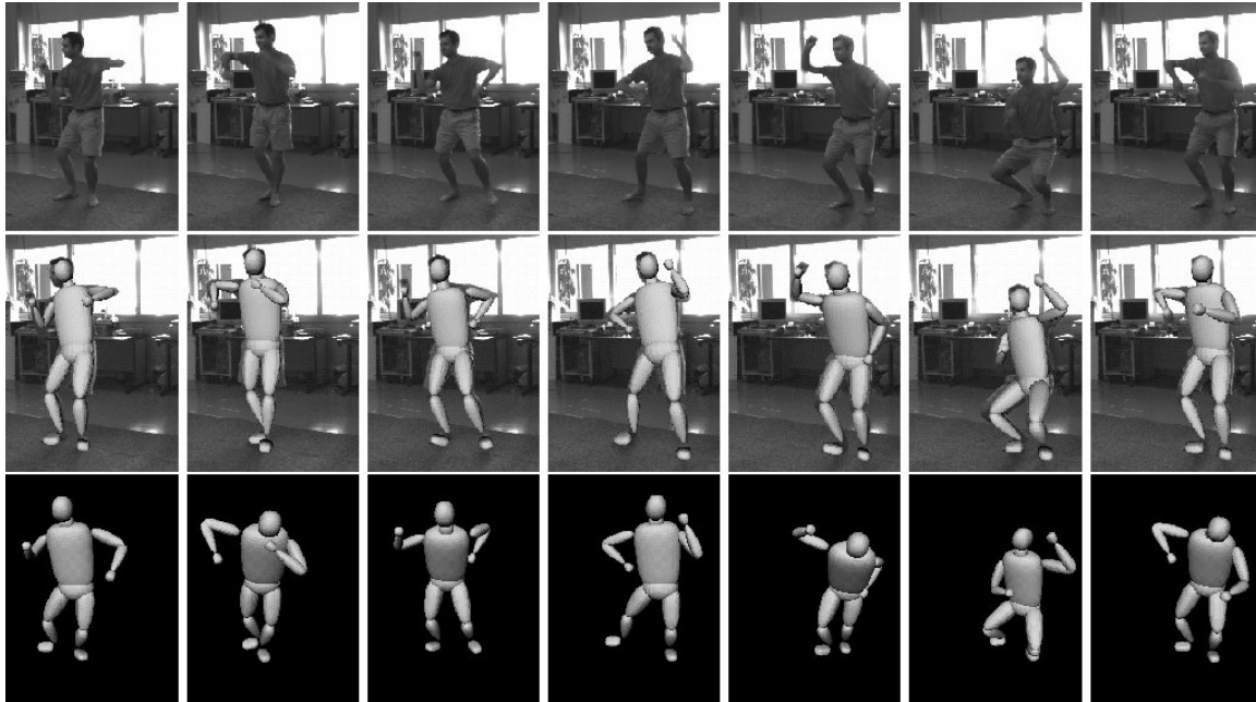
Figure 13. Tracking results for a 4 second dance sequence, using our kinematic jump based monocular human tracker. First row: original images. Middle row: 2D tracking results showing the model-image projection of the best candidate configuration at the given time step. Bottom row: the corresponding 3D model configuration rendered from above. Note the good model image overlap and the realistic quality of the reconstructed 3D poses.
