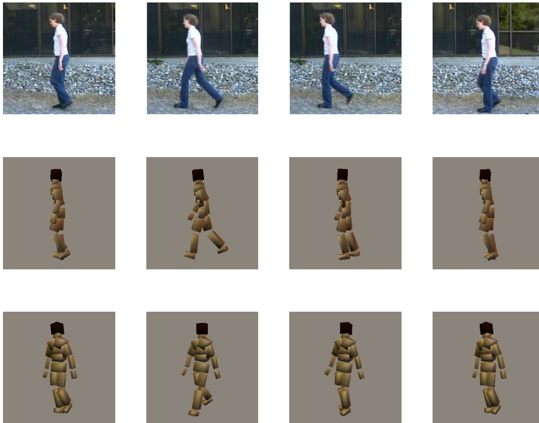
Figure 17. 3D poses reconstructed from some real images (part of a test sequence from http://www.nada.kth.se/~hedvig/data.html ). The middle and lower rows show the pose estimates from the original viewpoint and from a new one. The last two columns illustrate limitations of the current implementation. In the third column, a noisy silhouette causes slight mis-estimation of the lower right leg, while the final column demonstrates a case of left-right ambiguity in the silhouette.
