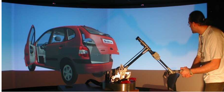
Figure 22. Direct immersive manipulation with haptic device Virtuose 6D .
