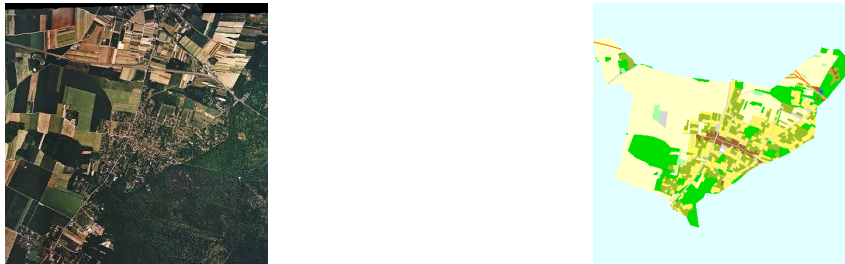
Figure 5. Image registration for the evaluation of retrieval systems. Left: mosaicked aerial image data; right: registered ground truth classification.
