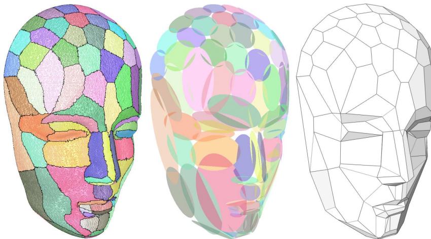
Figure 4. Variational Shape Approximation: Through repeated error-driven partitioning (left), we find a set of geometric proxies (represented as ellipses, center) providing a concise geometric description of an input triangulated surface (62K triangles) by efficiently capturing the anisotropy of the initial model; notice the presence of disks on near-spherical regions, and stretched ellipses on near-parabolic regions. These proxies are then used to construct an approximating polygonal mesh (right). No user interaction, parameterization, or differential estimates have been used; total processing time: 3s.
