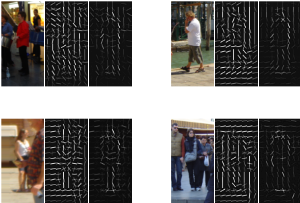
Figure 23. An illustration of the image information encoded by the HOG based detectors. In each triplet, we display from left to right: (1) the input image; (2) the corresponding HOG feature vector (only the dominant orientation of each cell is shown); (3) the orientations that dominate the descriptor output (obtained by multiplying the feature vector with the weights learned for the linear SVM). Inspection shows that for an appropriate choice of descriptor parameters, the SVM is able to map positive example images to a set of canonical edges corresponding to human contours.
