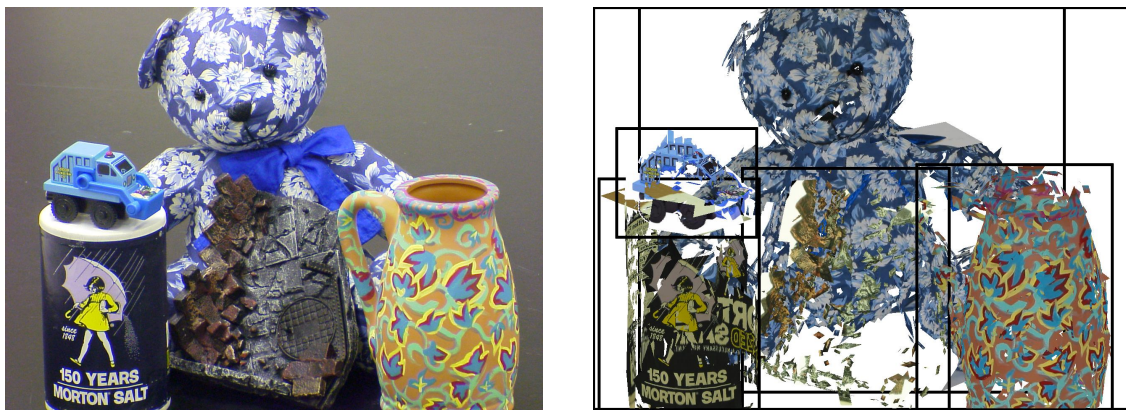
Figure 19. Results of a recognition experiment. Left: A test image. Right: Instances of five models (a teddy bear, a doll stand, a salt can, a toy truck and a vase) have been recognized, and the models are rendered in the poses estimated by our program. Bounding boxes for the projections are shown as black rectangles.
