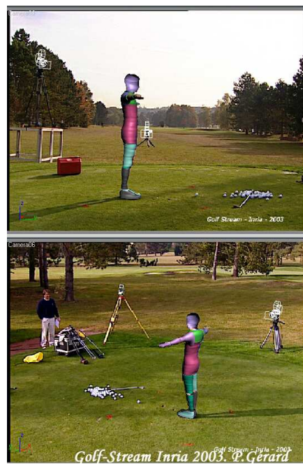
Figure 2. Skin reconstruction using several views
