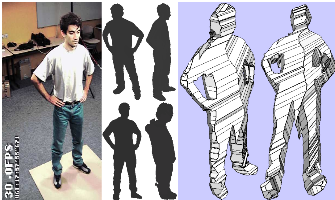
Figure 9. Real time reconstruction of a person with 4 cameras and the exact visual-hull approach.
