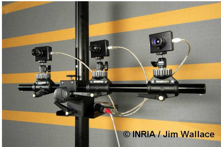
Figure 2. These three cameras are linked to the PC cluster through the IEEE 1394 bus protocol and they are synchronized with all the other cameras forming the acquisition setup.
