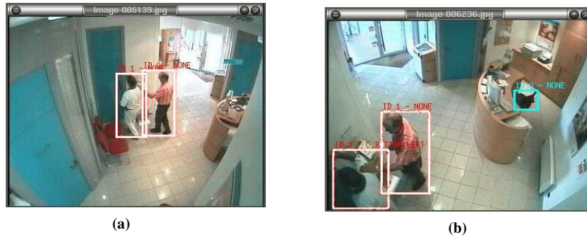
Figure 15. Images (a) and (b), taken with 2 synchronized cameras with overlapping field of view working in a cooperative way, illustrate a bank agency monitoring system detecting an abnormal “bank attack” scenario.
