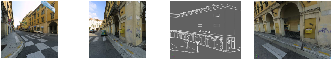
Figure 12. Two faces of a panorama cubemap used for image modeling. Wireframe of the resulting model and a view with extracted textures.
