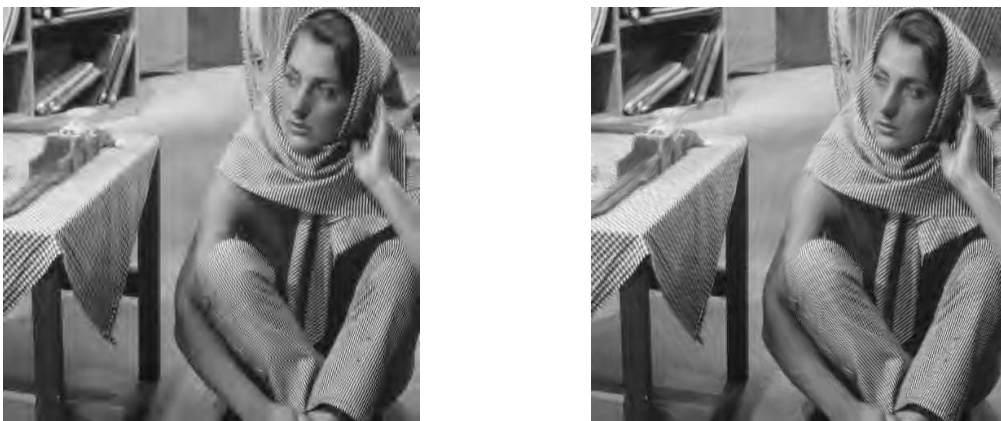
Figure 7. Images coded/decoded with a separable wavelet transform (left, PSNR=27.25dB) and with an oriented wavelet transform (right, PSNR=28.50dB) at 0.3 bpp.
