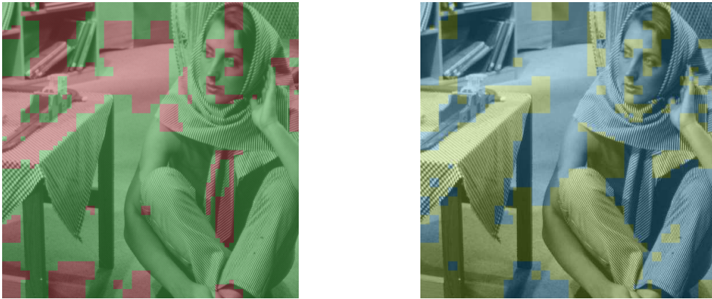
Figure 6. Maps of filtering orientations obtained with quad trees. The image on the left represents the horizontal (red) or vertical (green) filtering directions for the first decomposition level. The image on the right represents the diagonal '/' (blue) or antidiagonal '\' (yellow) filtering directions for the second decomposition level.
