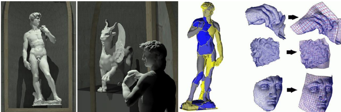
Figure 5. Left: results of our Discrete Master Element method for applying Finite Element Modeling methods to finely tessellated models; Right: construction of the wavelet basis attached to the object (mesh partition and extrapolation).
