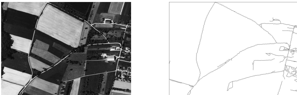
Figure 8. Left: aerial image (© French National Geographic Institute (IGN)); right: road extraction result
