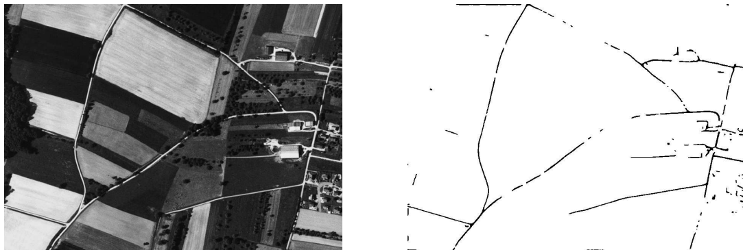
Figure 14. Left: an aerial image of a road network (© French National Geographic Institute (IGN)); right: the result of road network extraction with the phase field model.
