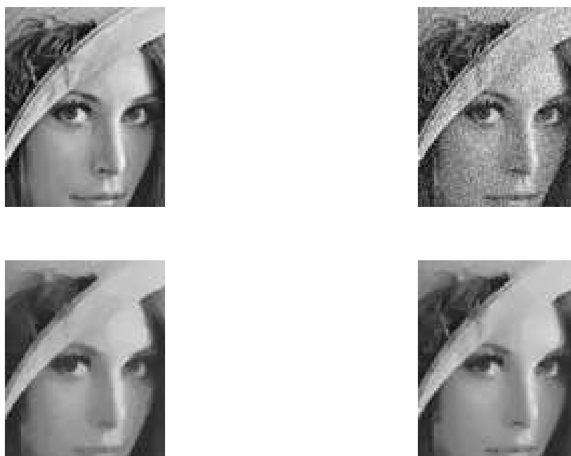
Figure 12. Top-left: original image; top-right: image with additive white uniform noise; bottom-left: restored image using the Rudin-Osher-Fatemi model; bottom-right: restored image with the proposed model.
