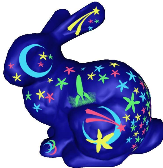
Figure 24. The Stanford bunny is textured using texture sprites. Each clip-art (stars, moon, rocket) are individual sprites that can be animated or generally modified independantly. Yet, rendering of the textured bunny is achieved at high frame-rate (e.g., 60 Hz).
