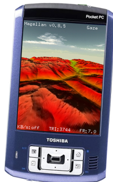
Figure 7. Real-time navigation in the Puget Sound terrain model made of 8 million of points on PocketPC.
