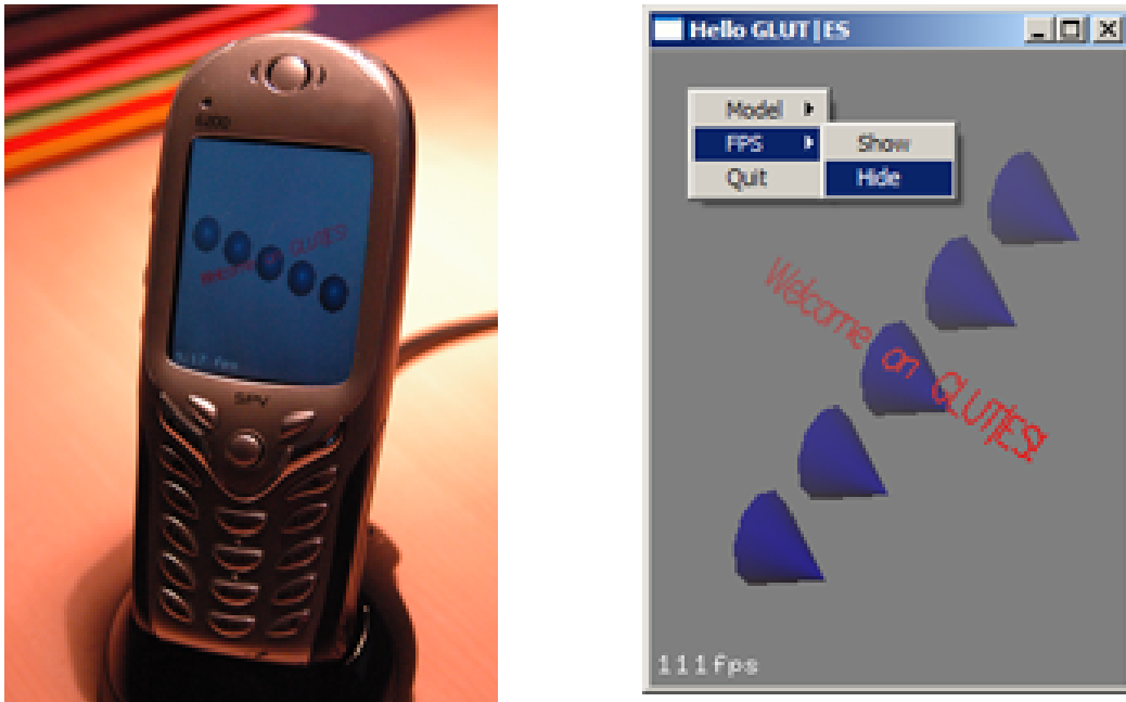
Figure 1. A sample application based on GLUT|ES and running on a Smartphone and a PocketPC.
