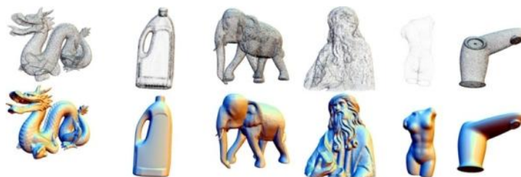
Figure 4. Different point clouds and their automatic conversion in subdivision patches for visualization.
