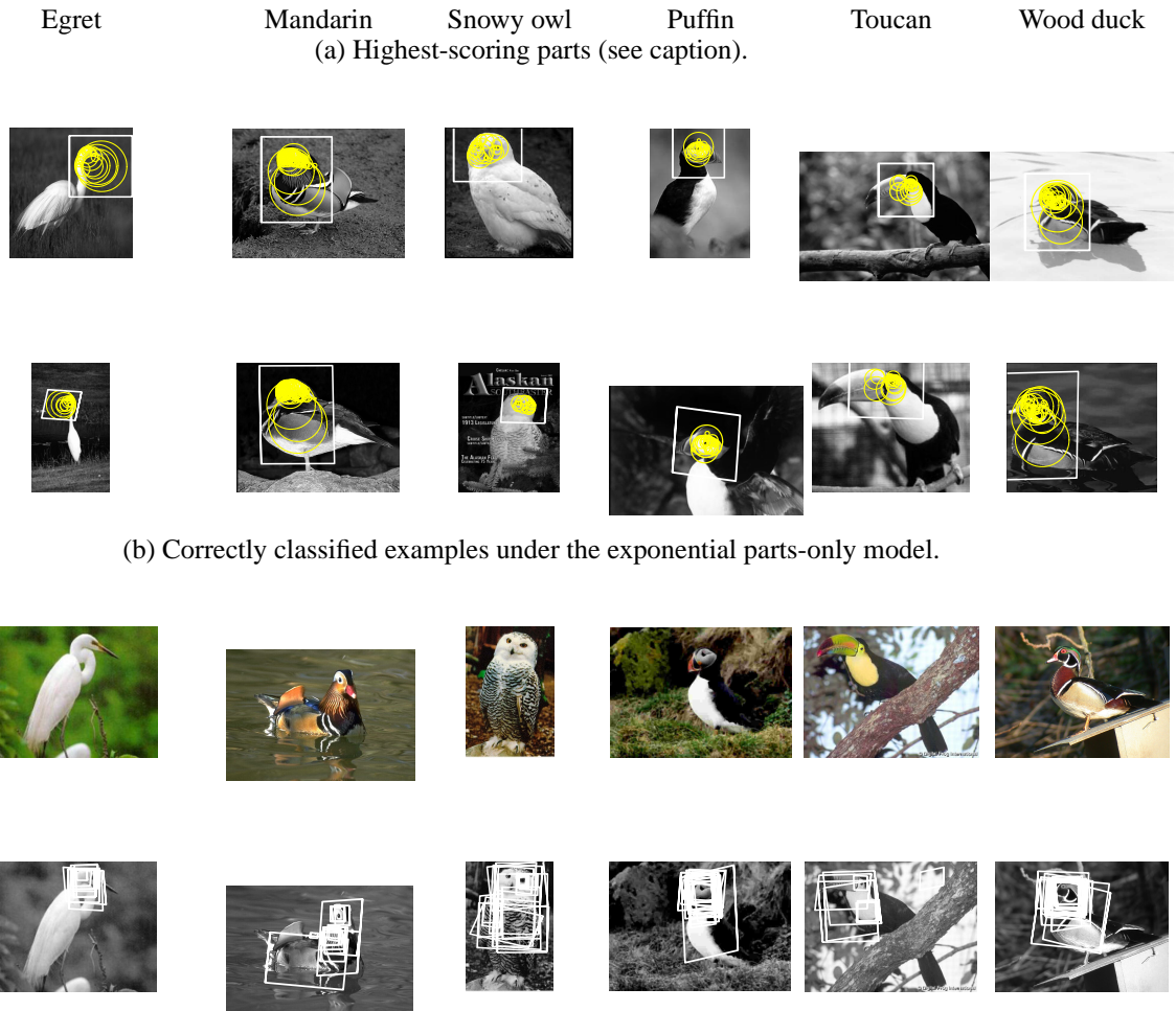
Figure 11. Semi-local parts – results on Birds database. (a) First and second rows: the highest-scoring part for each class superimposed on the two original training images. (b) A successfully classified image for each class, showing the original test image (top), and the image with the bounding boxes of all of the detected class part instances superimposed (bottom). Notice that localization is fairly good for mandarin and wood ducks (the head is the most distinctive feature). The owl parts are more prone to false positives but they do still capture the salient characteristics of the class: the head, the eye, and the pattern of the feathers on the breast and wings.
