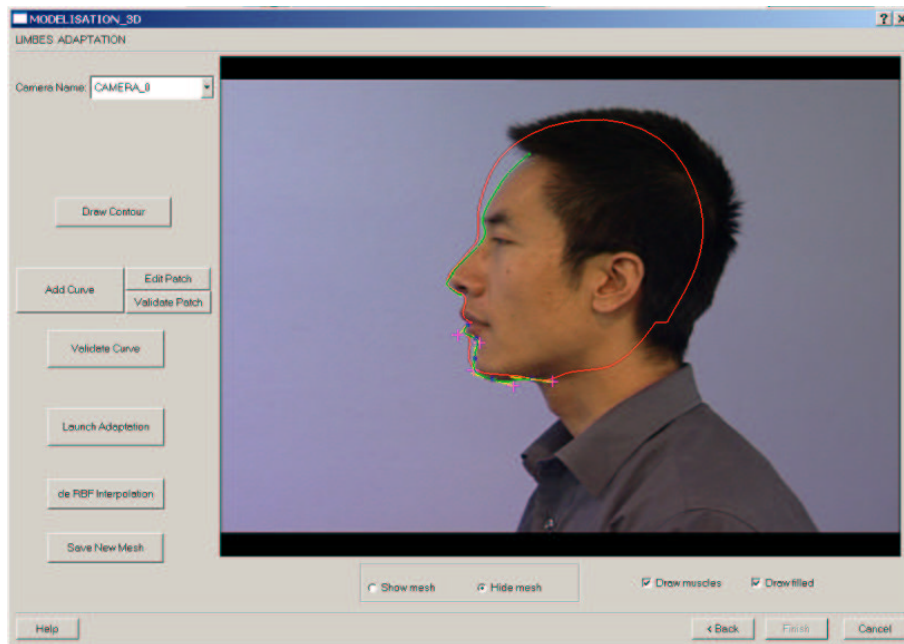
Figure 5. Adaptation of the model limbs (in red) to the Bezier curves (in green)
