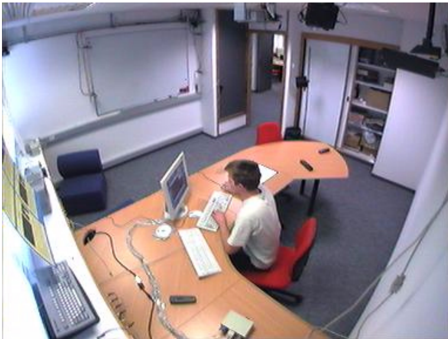
Figure 4. The augmented meeting environment is an office environment equipped with a microphone array, wireless lapel microphones, a wide angle surveillance camera, five steerable cameras, and three video-interaction devices.
