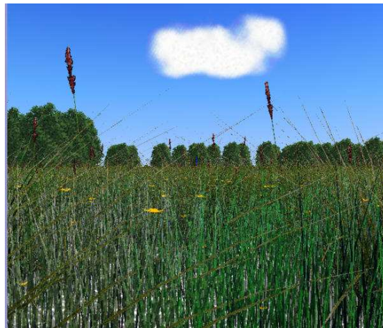
Figure 1. Plausible rendering of an outdoors scene containing points, lines and polygons [28], representing a scene with trees, grass and flowers. We can achieve 7-8 frames per second compared to tens of seconds per image using standard polygonal rendering.
