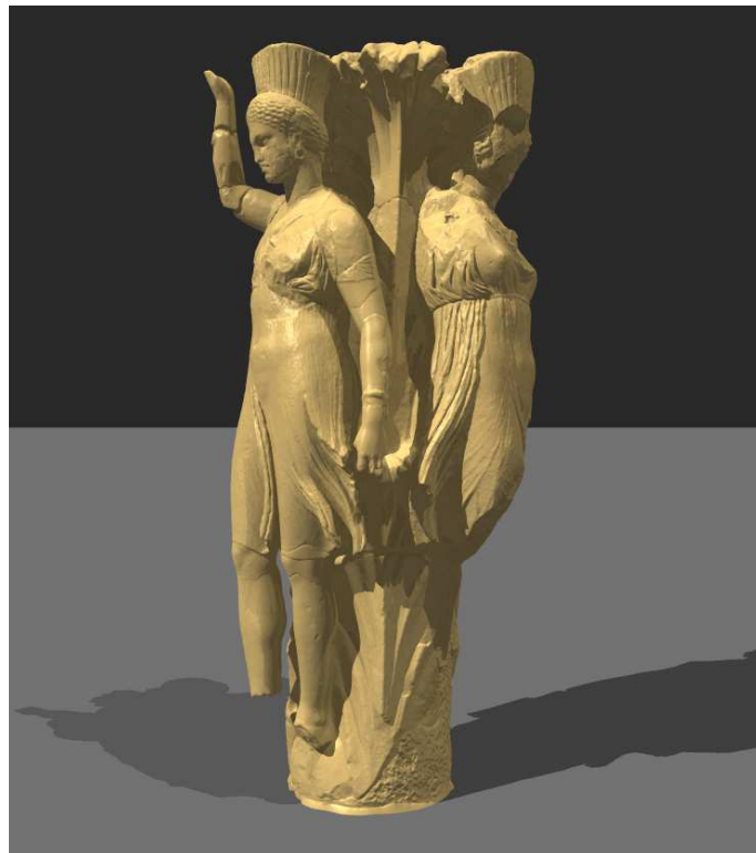
Figure 9. The dancers model: 49,500,000 input points level 11 of the octree, and raytraced at image resolution 1670x3400. Rendering this image required about 4 hours. (Two light sources, and maximal reflexion depth of 2.)
