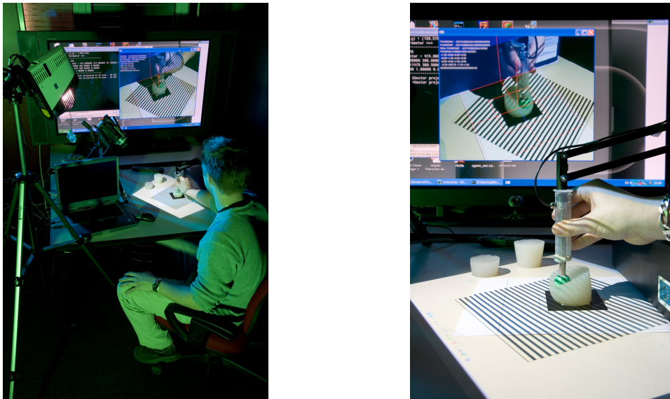
Figure 6. Left: our device for real-time capturing of external forces applied on an object. Right: A closer look at the system.
