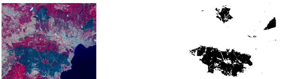
Figure 8. Left: SPOT 5 image (©CNES); right: Extracted burnt areas (only 4% of error compared to ground truth).
