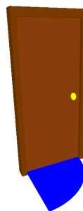
Figure 42. An influence surface (in blue) indicates the area to avoid while opening a door.
