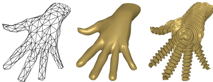
Figure 6. Controllable Adaptive Real-Time Mesh Refinement. From left to right: the on-CPU coarse mesh (576 triangles), an adaptive refinement topology generated in a single pass on the GPU (290000 triangles) and a procedural displacement applied on it (same pass).
