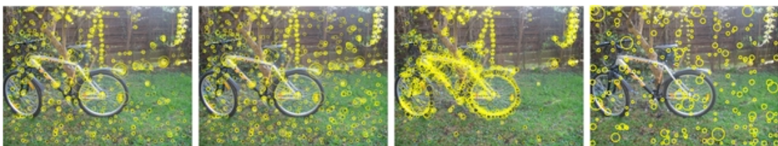
Figure 4. Examples of different sampling methods. (1) Harris-Laplace (HL) with a large detection threshold. (2) HL with threshold zero – note that the sampling is still quite sparse. (3) Laplacian-of-Gaussian. (4) Random sampling
