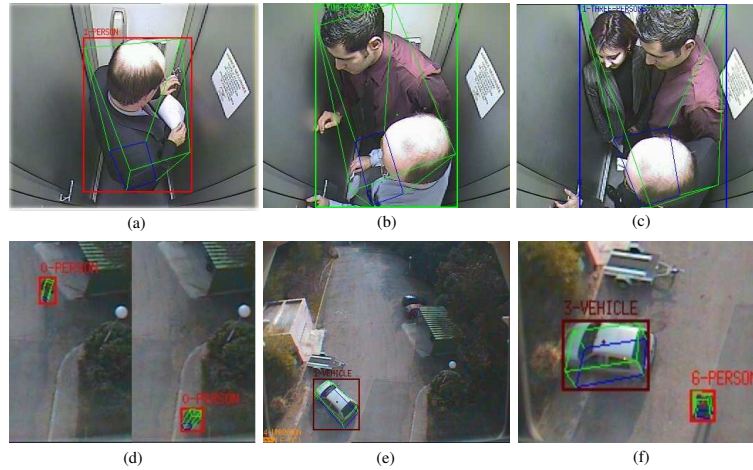
Figure 7. Resulting frames for the proposed classification approach. Top frames show the results for people counting application in a locked chamber: an instance of the class PERSON (figure (a)), of the class TWO-PERSONS (figure (b)), and of the class THREE-PERSONS (figure (c)) have been detected. Bottom frames show the results for a parking lot application: in figure (d) an instance of the class VEHICLE have been detected, in figure (e) the same PERSON at two different frames is correctly classified, and in figure (f) an instance of the class PERSON and other of the class VEHICLE is correctly classified at the same frame.
