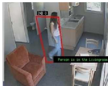
Figure 11. Recognition of the primitive state “Inside_zone” in GER'HOME laboratory. A text message “Person is in the Livingroom” is displayed on the screen when the event is recognized.
