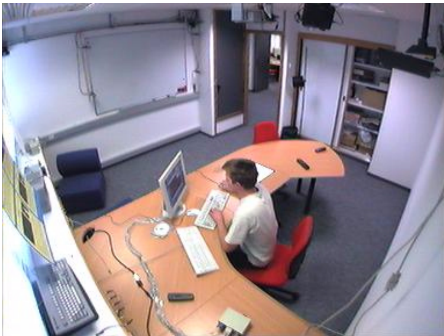
Figure 5. The augmented meeting environment is an office environment equipped with a microphone array, wireless lapel microphones, a wide angle surveillance camera, a panoramic camera, six steerable cameras, and two camera-projector video-interaction devices.
