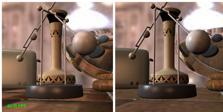
Figure 7. Left, a frame of an interactive sequence using our method, running at 82fps. Right, a ray-traced image (5 seconds to compute one frame)
