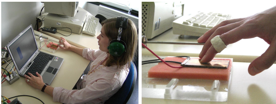
Figure 9. The tactile stimulator and the experimental test bench
