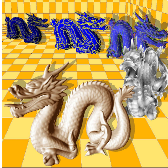
Figure 9. Geometry Textures : We developed algorithms to convert a scanned mesh into a set of height fields, and algorithms to display these height fields in real-time on the GPU.
