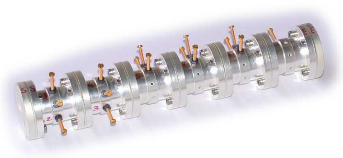
Figure 2. Picture of a 6-cavities dual mode filter. Each cavity (unless the last one) has 3 screws to couple the modes within the cavity, so that there are 16 quantities that should be optimized. Quantities like the diameter and length of the cavities, or the width of the 11 slits are fixed in the design phase.
