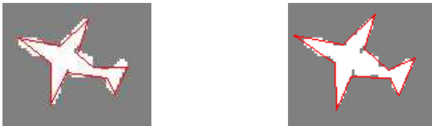
Figure 12. Naive initialisation (left) and convergence (right) of the polygonal approximation algorithm on the shadow of an aeroplane.
