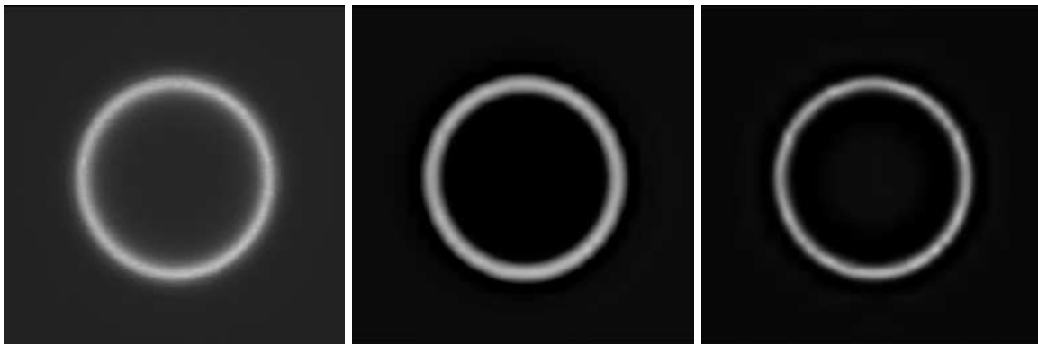
Figure 26. Restoration of an image of a shell. Left: raw data; centre: restored images using method 1 (denoising + deconvolution); right: restored images using method 3 (combined approach).
