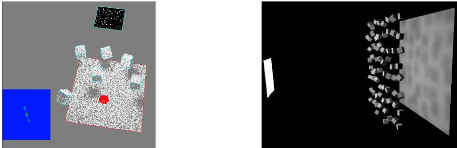
Figure 1. Left: a simple configuration where blockers are the cause of high frequencies of the lightfield onto the receiving surface. The blue square shows a clue of what the spectrum in space and angles looks like. Right: from the spectrum, a correct sampling density for the image is produced, which allows to allocate an optimal amount of cpu time to the computation of the shadow onto the receiver.
