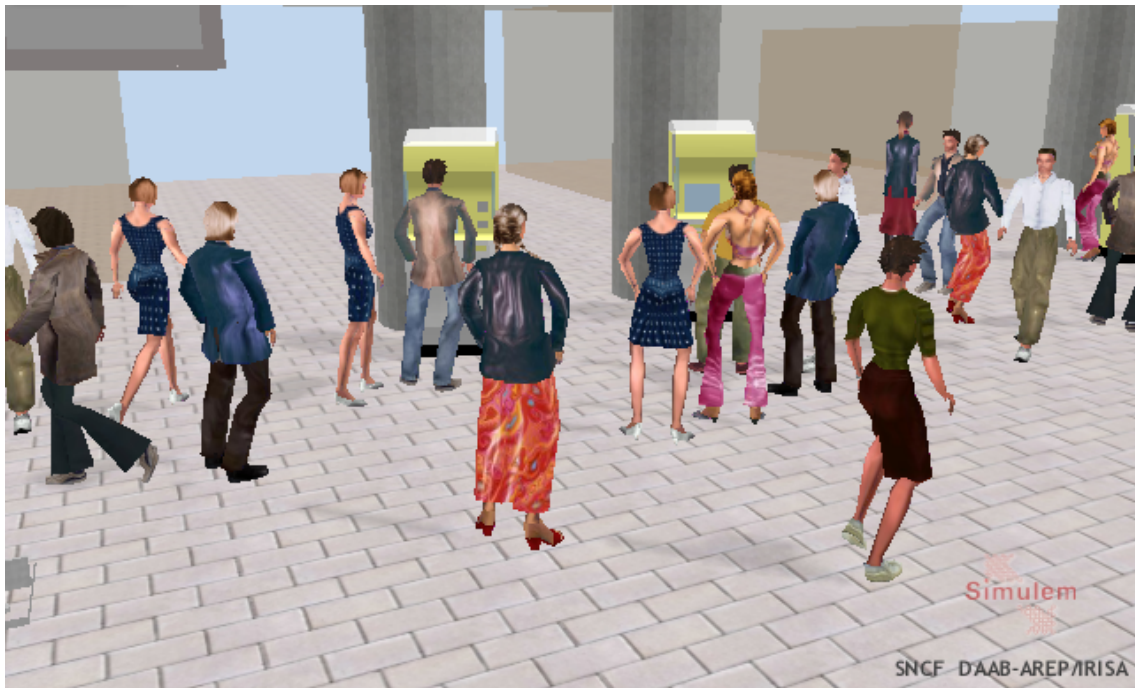
Figure 40. Example of the 3D graphical output of SIMULEM. Here we can see some waiting queue formations in front of ticket selling machines, while other people walk to reach other goals.
