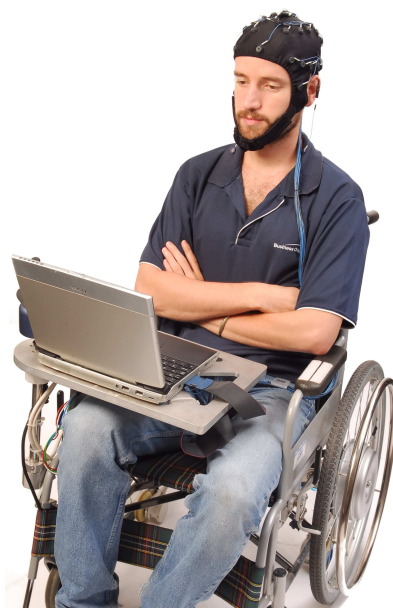
Figure 23. Photograph of the prototype brain controlled wheelchair based on a standard powered wheelchair. A laptop is connected in between the joystick and the power drivers, and rotary encoders mounted on glide wheels fixed below the seat are used for odometry.
