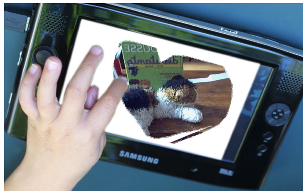
Figure 11. Sketchcam allows children to capture and interact with the world through annotations.
