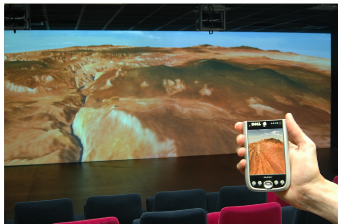
Figure 4. Adaptive rendering of the same terrain on a PocketPC and on a virtual reality center using Elkano.
