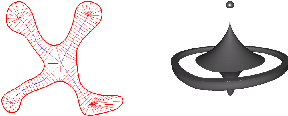
Figure 24. A smooth skeleton extracted with our technique (left). Since it is combined with a better sampling of the silhouette, our system creates models with better quality meshes (right).
