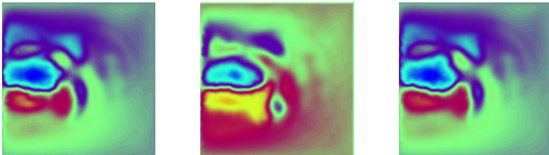
Figure 5. BFN on a shallow-water model: data assimilation period = 1 month, forecast period = 3 months; model states at the end of the forecast period: true state (left), no assimilation (center), BFN assimilation (right).
