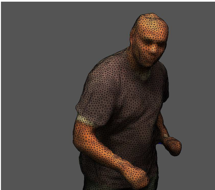
Figure 1. One of our main goals is to develop methods for building realistic 3-D visual content from multiple images and multiple videos. A set of 30 cameras that are precisely calibrated and finely synchronized (top) gather images and videos which are subsequently processed to produce highly realistic visual content, such as the 3-D texture mapped onto a surface (a mesh).
