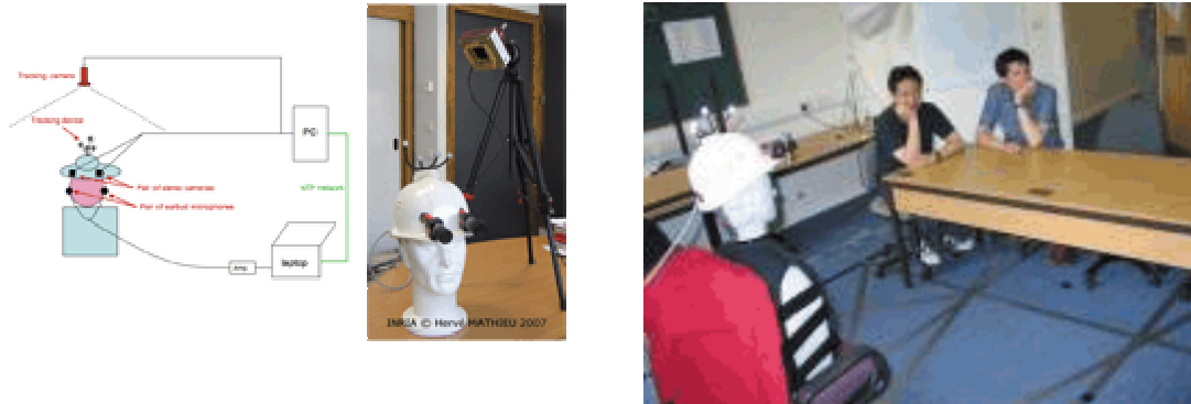
Figure 5. Recently we gathered an audio-visual set of data that consists in stereo image pairs and binaural recordings. An audio-visual sensor consisting in a pair of cameras and a pair of microphones can be mounted on a person's head or on a mannequin head. In addition we recorded the position and orientation of the head.
