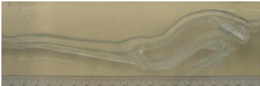
Figure 1. Phantom built by rapid prototyping from the surface mesh of the computational model of the carotid artery network.
