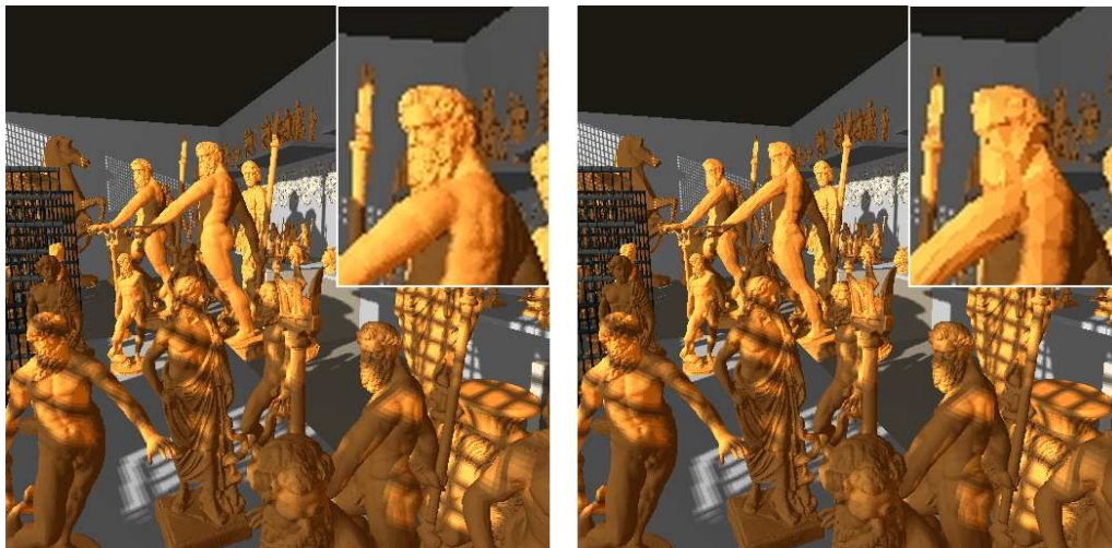
Figure 7. The rendering of a complex museum scene with our pipeline calibrated for a 512x512 Resolution image (left) and with a distance based LOD selection (right). The zoomed insets clearly show the difference in the choice of LOD
