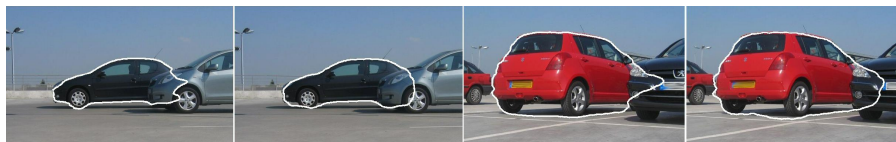
Figure 8. Segmentation of a Peugeot 206 (left) and a Suzuki Swift (right) with data term only (first images) and with shape prior (second images).
