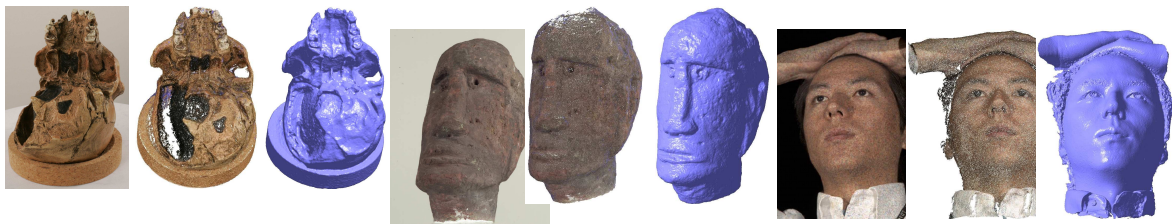
Figure 1. Sample reconstructions using the PMVS software. In each case, one of the input image is shown, along with views of texture-mapped reconstructed patches and shaded polygonal surfaces.
