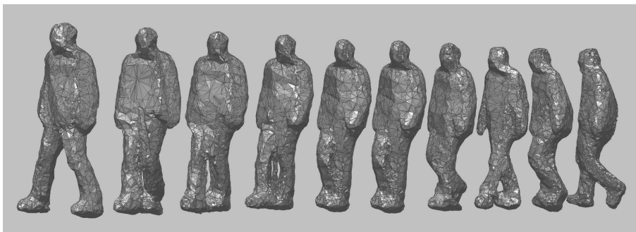
Figure 3. Sample frames of the spatio-temporal visual hull of a walking person.
