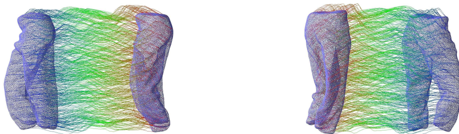
Figure 4. In our approach to motion capture, a polyhedral mesh deforms as its vertices are continuously tracked under locally rigid and globally nonrigid motion models. This is illustrated here with a mesh extracted from real data consisting of 8 synchronized video streams 155 frames long (White et al. , 2007). The mesh is shown from two different viewpoints in states 30 frames apart, along with the trajectories of a subset of its vertices (the translational motion is exaggerated for better visualization).
