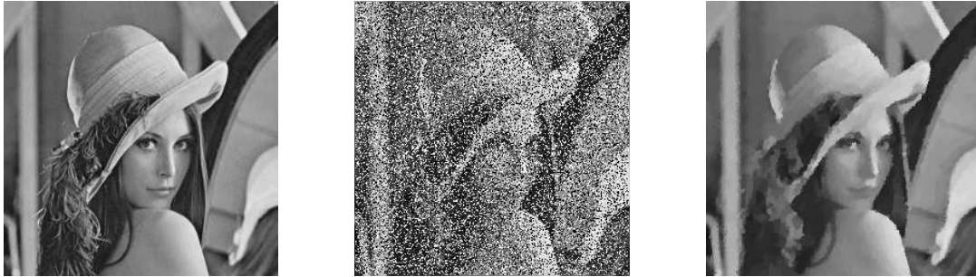
Figure 15. Left to right: original image; noisy image (salt and pepper 40%); image restored with a BV - L^1 model.
