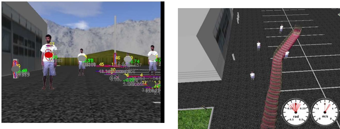
(a) An example of ridge segment tracking and TTC estimation in the camera image (red discs indicate a short TTC).
