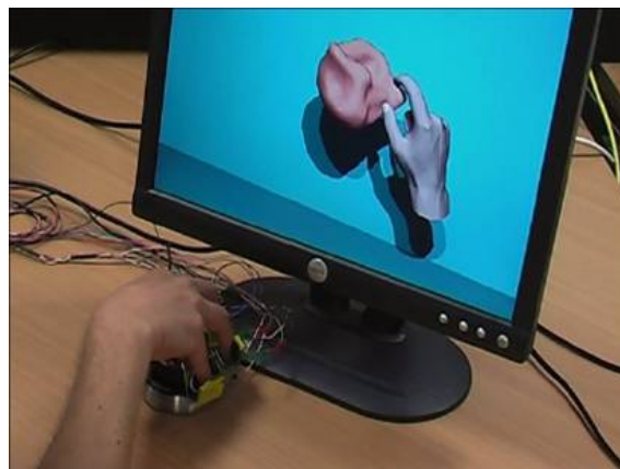
Figure 5. Hand-Navigator: a new device for interacting with virtual clay.
