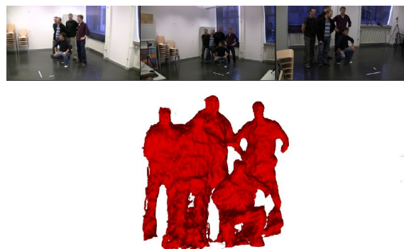
Figure 7. Result of modeling a multi-person scene from the silhouettes obtained from 3 calibrated views and a calibrated depth camera.
