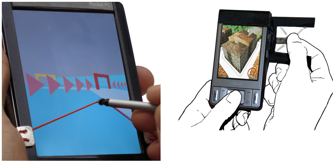
Figure 15. (a) 3D elastic control on a PDA for exploration of virtual cities. (b) 3D elastic control device on a PDA.
