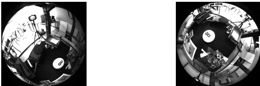
Figure 4. Visual servoing of a special sphere using a fisheye camera: initial image on the left and desired image on the right.
