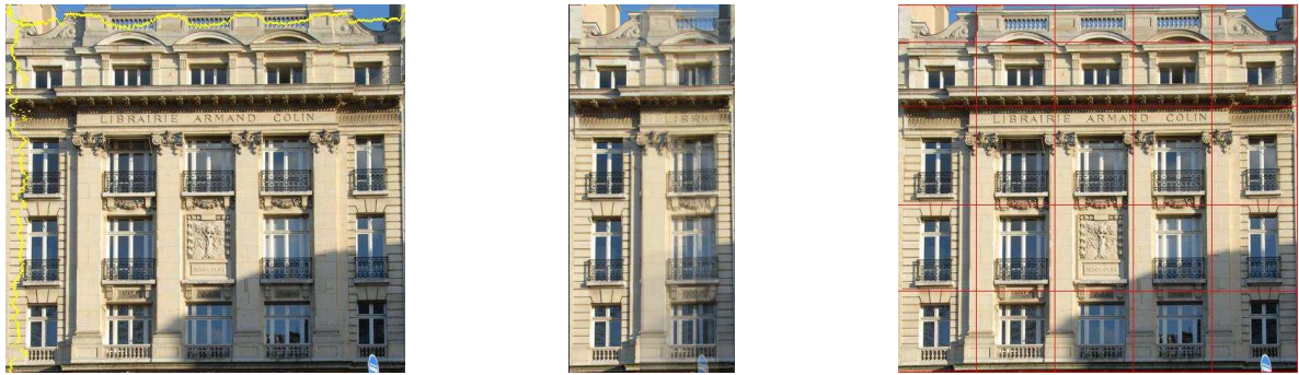
Figure 32. Left: Original image with global edge profile in yellow. Middle: Tile templates. Right: Subdivision based on edge profile and GMI (splitting lines in red).
