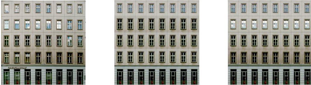
Figure 36. Left: Original image. Middle: Reconstructed 2D facade image before optimization. Right: Reconstructed 2D facade image after optimization.
