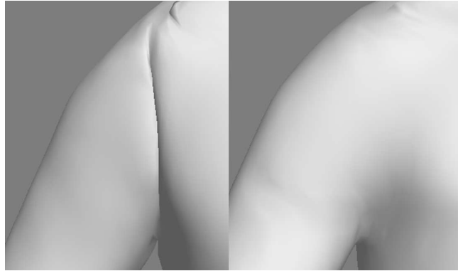
Figure 29. Difference between the case where we don't use B-splines to fit the curves (left) and the result when B-splines are used with d = 3 n = 35 (right).
