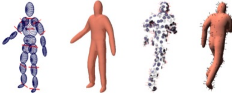
Figure 4. From left to right: A set of ellipsoids and their associated articulated implicit surface; Observations composed of 3D points and normals; the pose of the articulated model that fits the observations.
