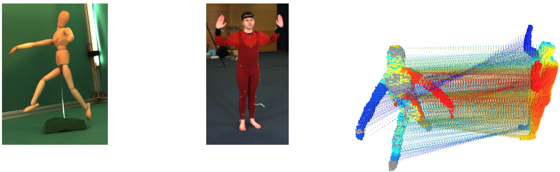
Figure 8. From left to right: A mannequin, a person, and their matched voxel representations.
