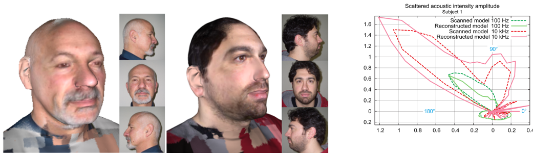
Figure 11. Left: Two results of processed heads and Right: Matching simulated HRTF measurements for a scanned model and a reconstructed model
